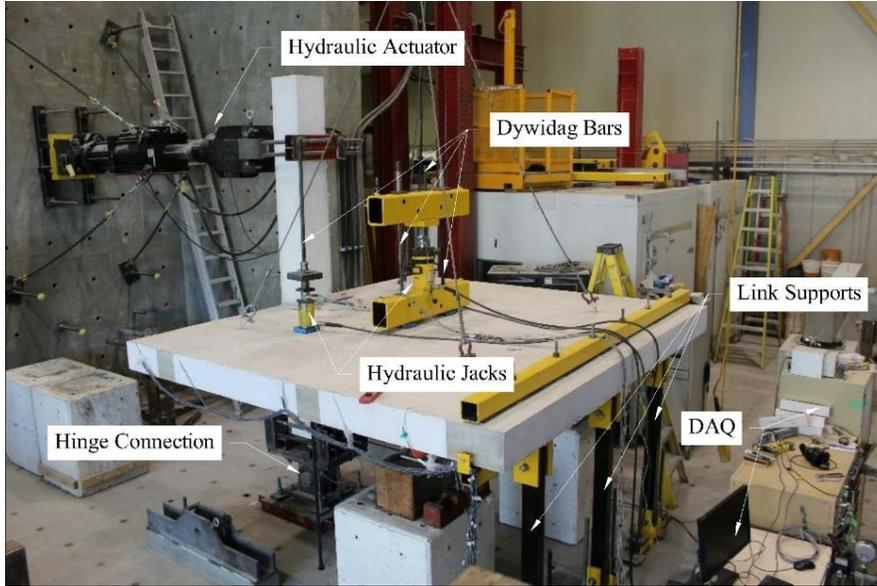
Figure 2. Test setup.
