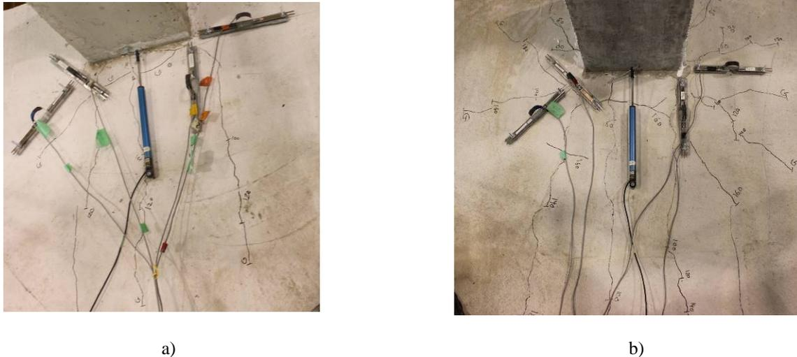
Figure 4. Cracking pattern after the application of gravity load: (a) connection E50, (b) connection E60.
