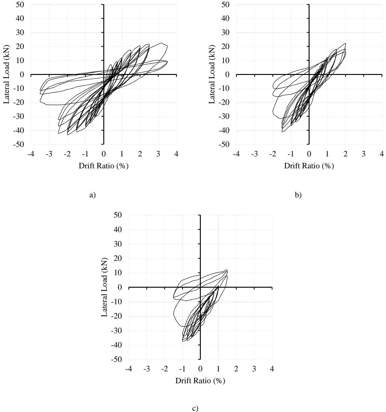
Figure 6. Hysteresis diagrams: (a) connection E40, (b) connection E50, (c) connection E60.
